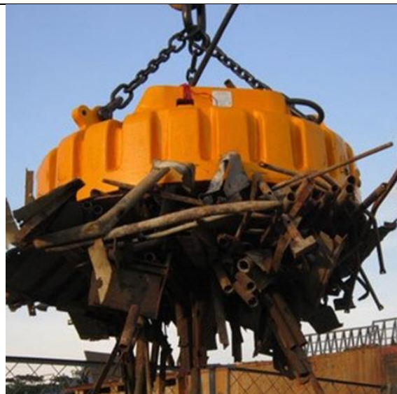
A crane with an electromagnet lifting scrap metal waste.
