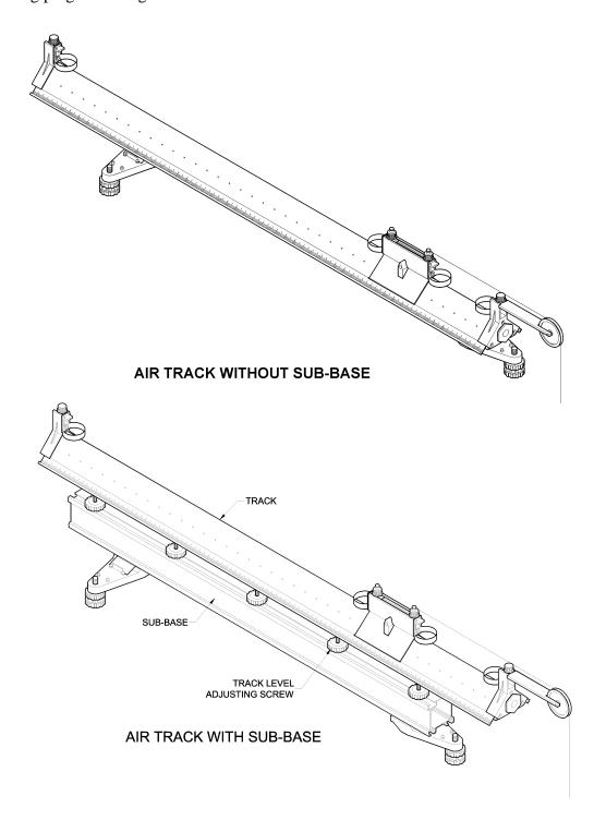
Sub Bases are used normally on long Air Tracks or where the track straightness must be exact. Sections of the track can be raised and lowered slightly by adjusting the special screws.
