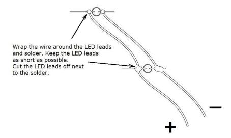
NOTE: If you are mounting the LEDs in a piece of plywood or plastic. You will need to drill 4.9mm holes to make the LEDs a press fit. Not all LEDs are exactly the same size so some LEDs will fit snugly while others will require some force to fit them into the hole. Do not drill the holes closer than 10mm apart or you may experience material between the holes breaking when you insert the LEDs.
